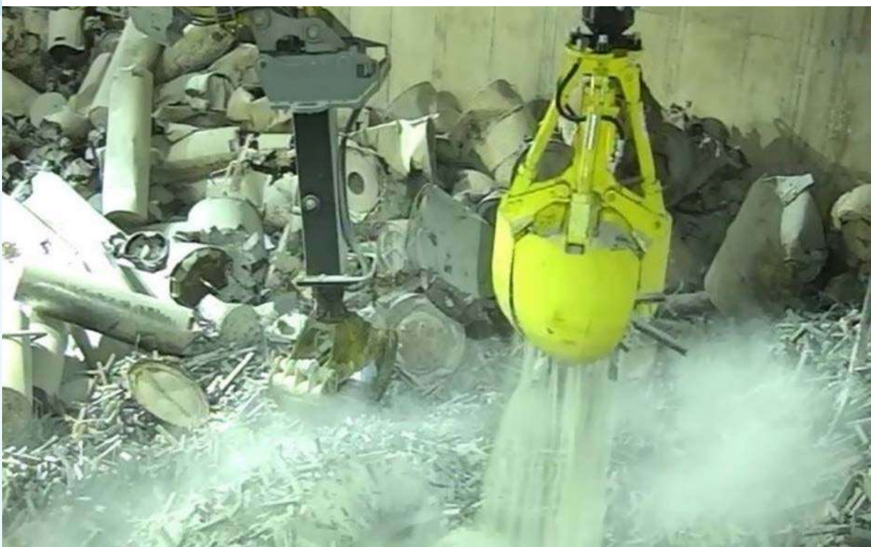
Figure 7: Retrievals of intermediate level waste from the subterranean vaults
