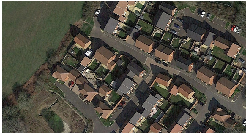
Figure 43: Example of recent development, elsewhere in UK, which should not be acceptable in Hermitage's rural context as it consists of regular building lines with minimum variations and lack of natural boundary treatments or vegetation along the edges.
