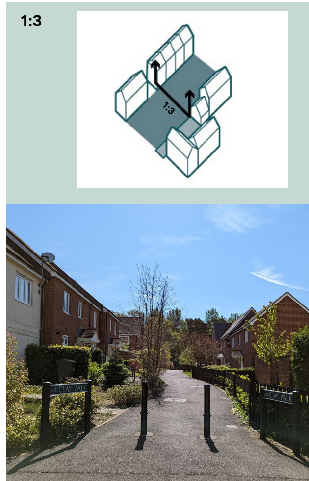
Figure 51: Local example of 1:3 enclosure, which is created by the footpath in combination with varied building setbacks and 2-storey buildings heights.
