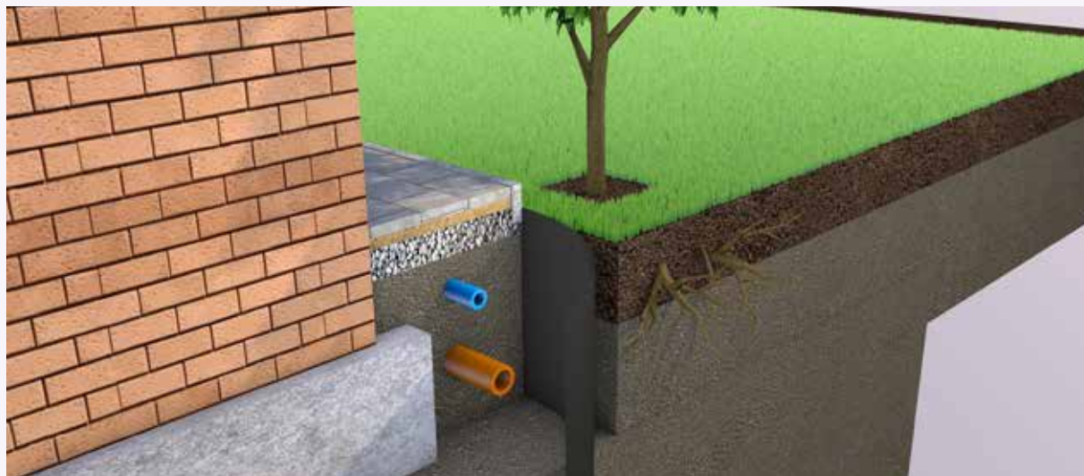
Figure 10 Root barriers prevent damage to paths and services by diverting root growth away from structures and services and into uncompacted soils.
